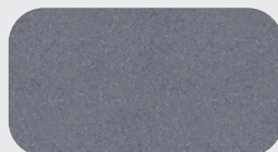
WEATHERED GALVALUME SR:0.30 E:0.79 SRI:27
