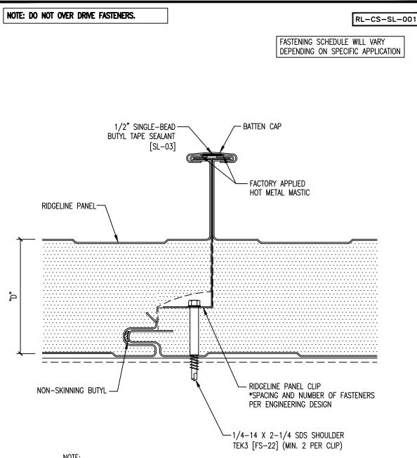
1. "D" = ROOF PANEL THICKNESS (AVAILABLE THICKNESS = 2.5, 3, 4, 5 OR 6)
