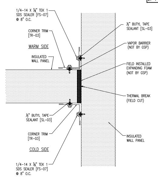
NOTE: FIELD CUT START PANEL AND ENDING PANEL AS REQUIRED AT CORNER TRANSITION. USE OF RECIPROCATING SAWS IS PROHIBITED
