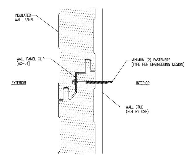
3/8" UNIFORM BEAD OF NON-SKINNING BUTYL SEALANT MUST BE APPLIED IN THE EXTERIOR FEMALE GROOVE. APPLYING SEALANT IN THE INTERIOR FEMALE GROOVE IS OPTIONAL DEPENDING ON VAPOR SEAL REQUIREMENTS
